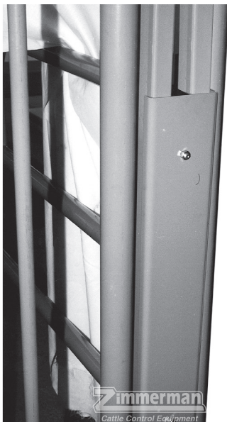
17. Attach mid-dividers using channel brackets.
