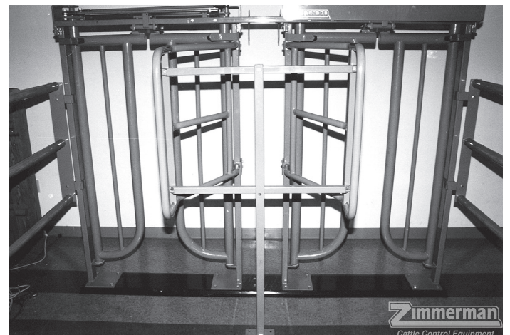
12. Bolt center support with cross bars to equipment rack sides. Loosen side clamp bolts and lower assembly onto floor. Tighten all side clamp bolts securing unit to stall posts. Bolt base plate of equipment rack center post to floor.
