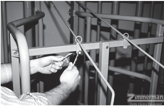
13. Pass both left and right release rods through their respective mounting brackets, and bolt brackets onto the top equipment rack cross brace.
