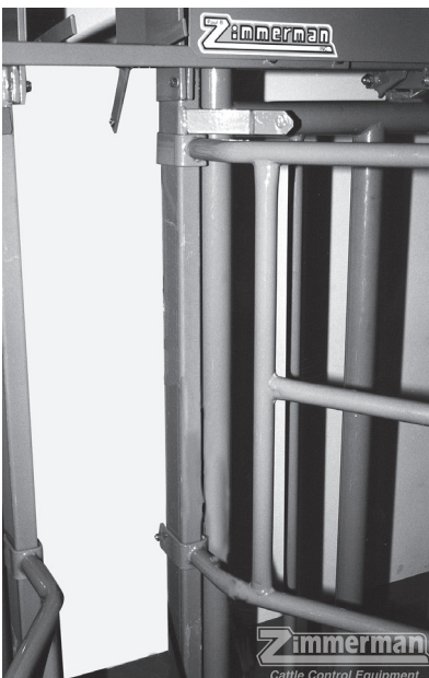
11. Position equipment rack fully at the top of the stall post. Tighten the top bolt (only) enough to hold rack in place. Additional adjustment will be done in next step.
